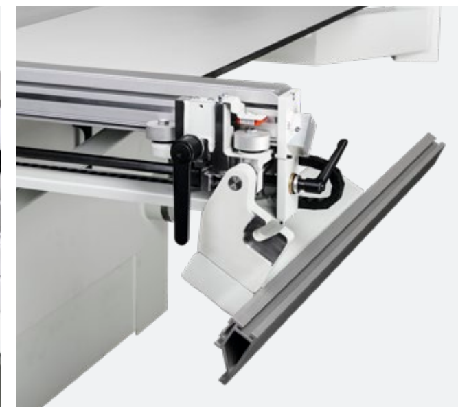
Tope paralelo T66 | T77, accionado mediante motor, abatible | Txx42
