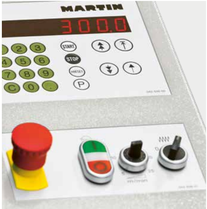
Avance regulable de forma continua 5 - 25 m/min | T4510
